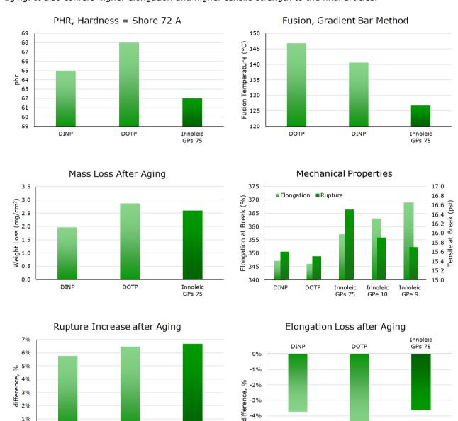
Hardness-adjusted compounds to 72 Shore A (s-PVC Resin with K value 65, CaZn thermal stabilizer 2phr) Formulations with petroleum-based plasticizers included 5phr of ESO as co-stabilizer Oven aging @ 100 °C, 12 air exchanges/hour, 168 hours
